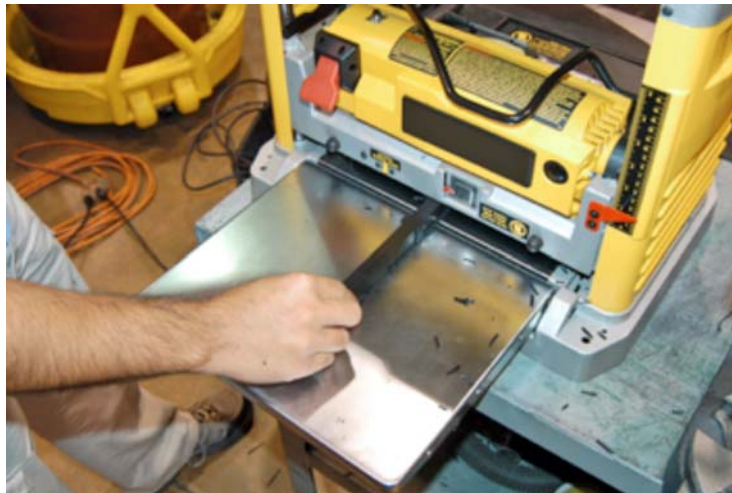
FIG. 7 Electric Planer for Side Bend Specimen Preparation
