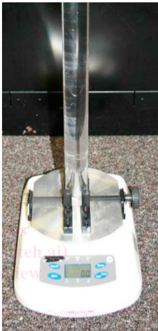
FIG. 1 Acrylic Rod Attached to a Torque Meter
