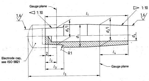
a) Type A: Adaptor with cooling hole open on one side
