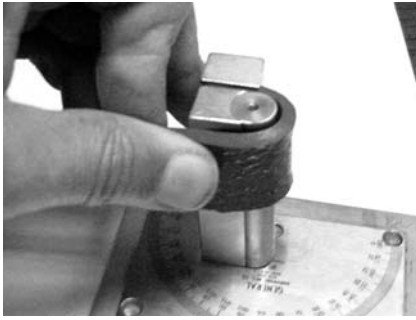
FIG. 3 Specimen Being Bent Around Mandrel
