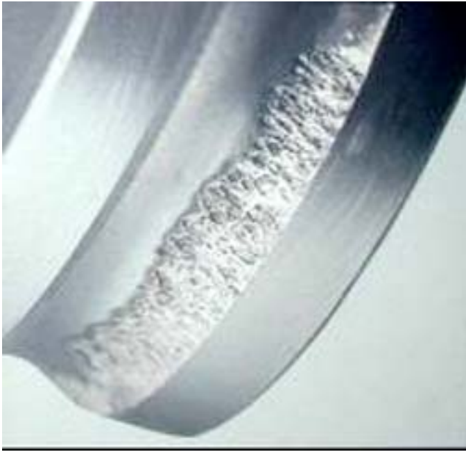
FIG. 2 Typical Bearing Spall
