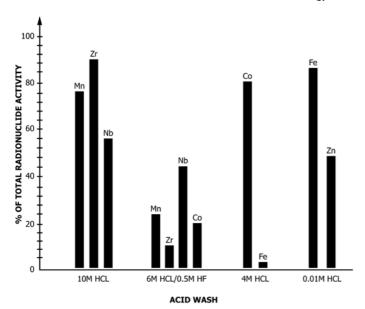
FIG. 1 Percent of Total Radionuclide Activity Removed Per Acid
