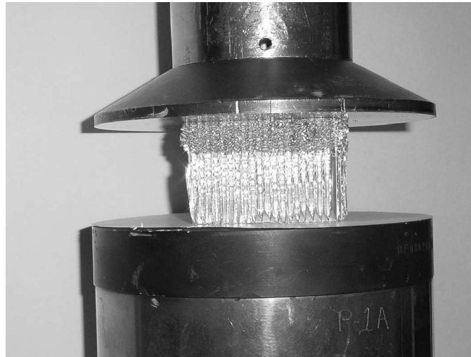
FIG. 2 Close-up of Specimen Between Loading Platens Being Crushed
