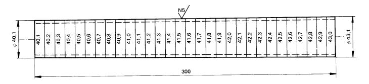
FIGURE 2 - Example of tapered plug gauge
