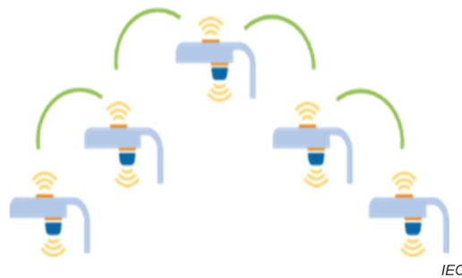
Figure 3 – Example of autonomous lighting system
