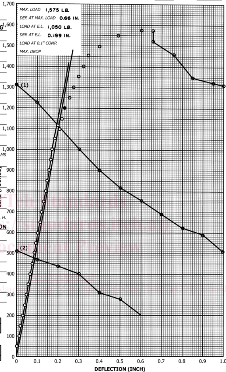
FIG. 5 Sample Data Sheet for a Manually Recorded Static Bending Test
