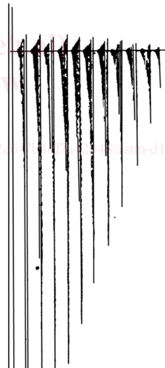
FIG. 12 Sample Drum Record of Impact Bending Test
