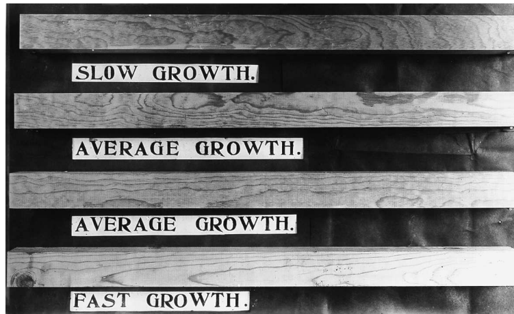
FIG. 2 Tangential Surfaces of Bending Specimens of Different Rates of Growth of Jeffrey Pine 22-in. by 22-in. by 30-in. (50 mm by 50 mm by 760 mm) Specimens
