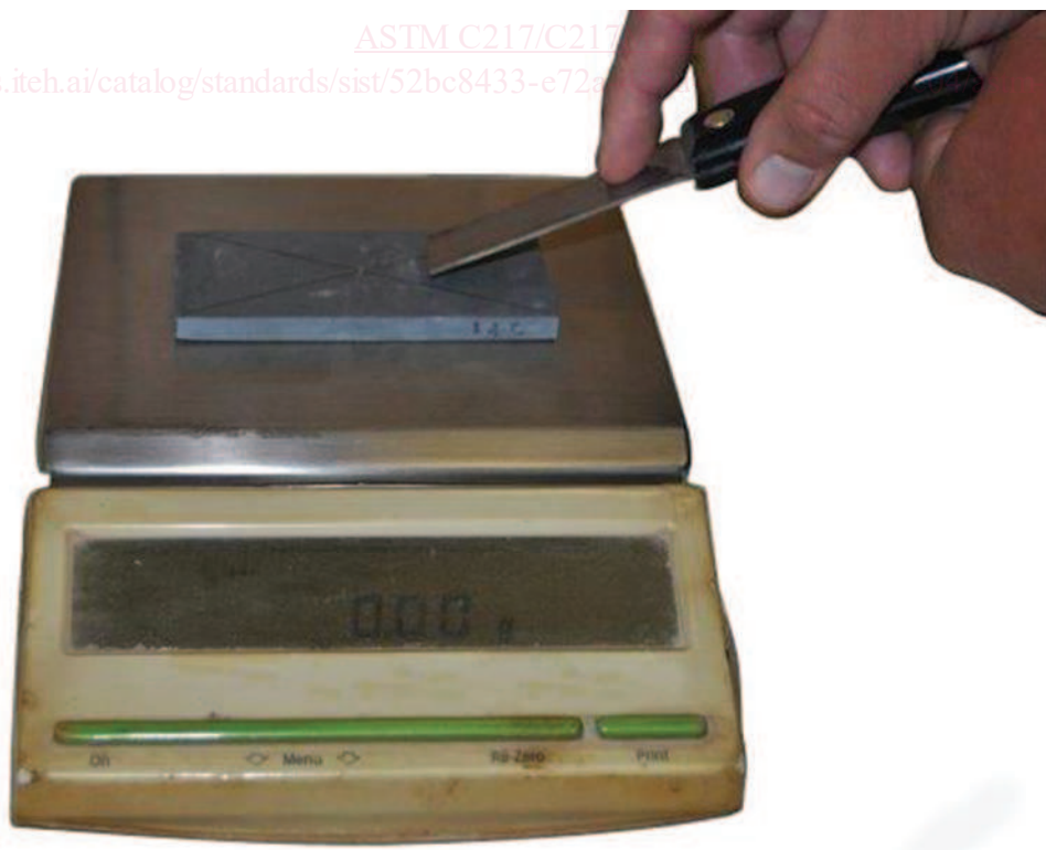
FIG. 3 Slate Specimen Prepared for Test with Hand Scraping
