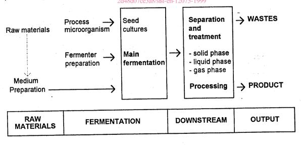
Figure 1 : Schematic diagram of a biotechnological manufacturing process
