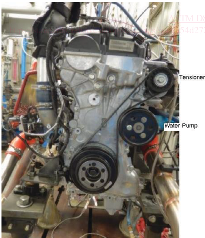
FIG. 3 Water-Pump Drive Arrangement
