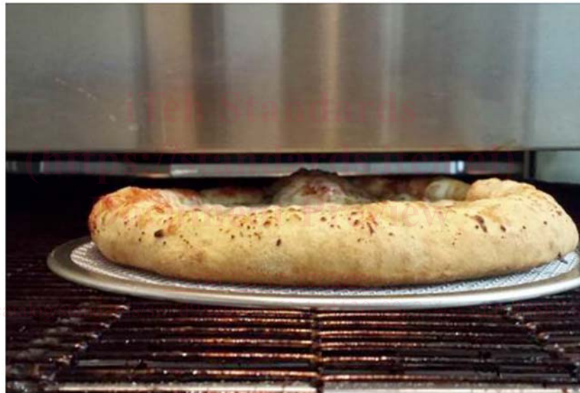
FIG. 3 Pizza Exit Must Clear Discharge Opening Without Touching
