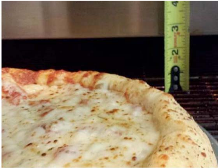
FIG. 2 Discharge Gap Minimum 2.25 in. (57.2 mm); Load Minimum Gap 1.25 in. (31.8 mm)
