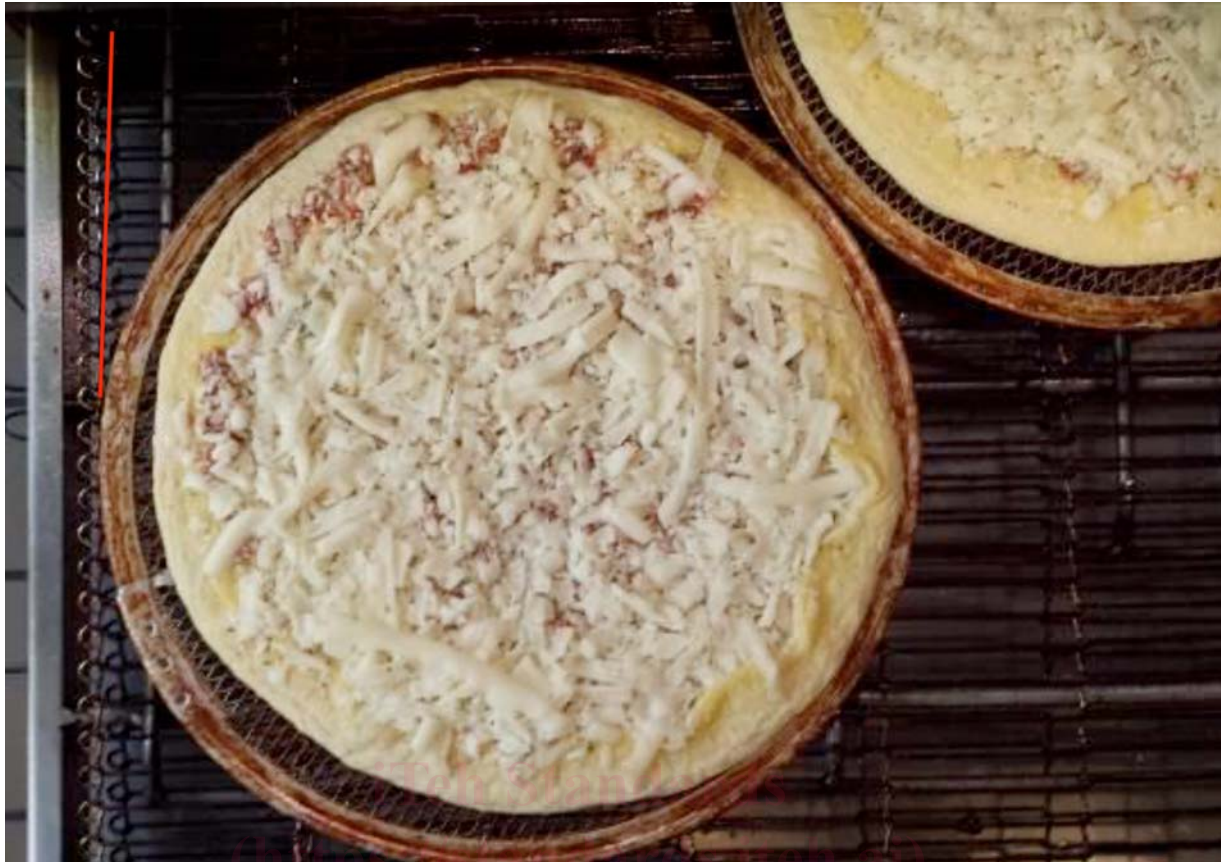
FIG. 5 Pizza screen edge aligned with inside knuckle of belt, result pizza approx. 1 in. from O.D. of belt width
