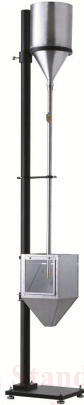
FIG. 1 Apparatus for Falling Sand Abrasion Test Apparatus
