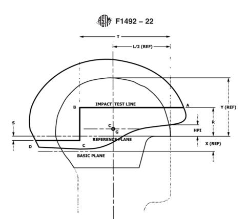
Note 1—The center of impact can be anywhere on or above the test line.
