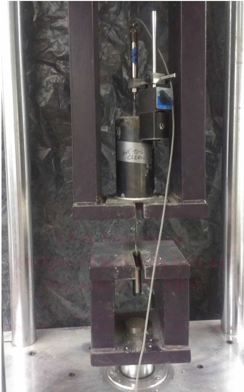
FIG. 1 Photo of Pullout Test Frame and Specimen as the Test is Being Conducted
