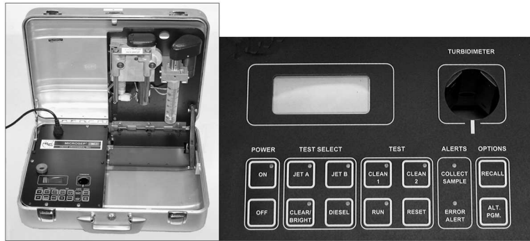
FIG. 2 Mark X Micro-Separometer and Control Panel
