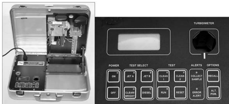
FIG. 2 Mark X Micro-Separometer and Control Panel
