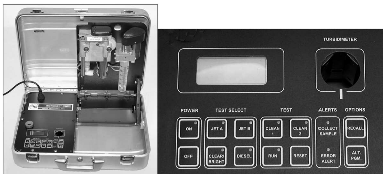
FIG. 2 Micro-Separometer Mark X and Control Panel
