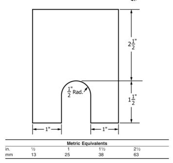
Note 1—The length of the keel block shall be 6 in. [150 mm].
