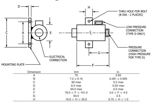
Note 1—Transducer housing (body) cross section is shown as circular. Any alternate cross section not exceeding 50 mm (2 in.) in width and 50 mm (2 in.) in height is acceptable.
