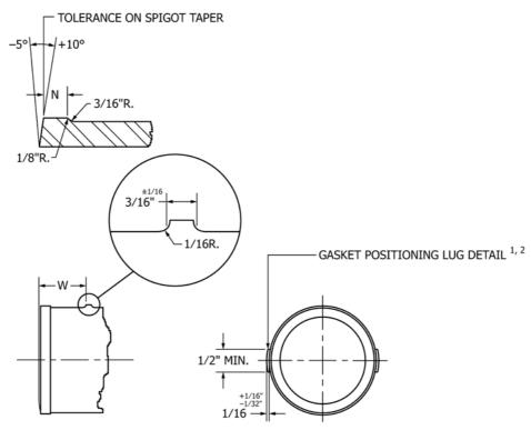
Note 1—These lugs and spigot beads are optional on all fittings. When a manufacturer chooses to utilize positioning lugs and spigot beads as illustrated above, these lugs and spigot beads shall be cast as illustrated or be continuous around the entire circumference.
