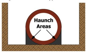
**haunching**—utilizing a shovel, spade, or other suitable tool to place and consolidate the bedding material in the haunch to (1) ensure the pipe will remain true to line and grade and (2) provide uniform circumferential support to the pipe, which is essential for the total load factor to be realized.
