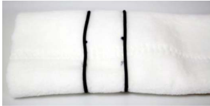
FIG. 1 SMHG O-rings on Tube at One End
