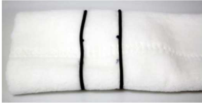
FIG. 1 SMHG O-rings on Tube at One End
