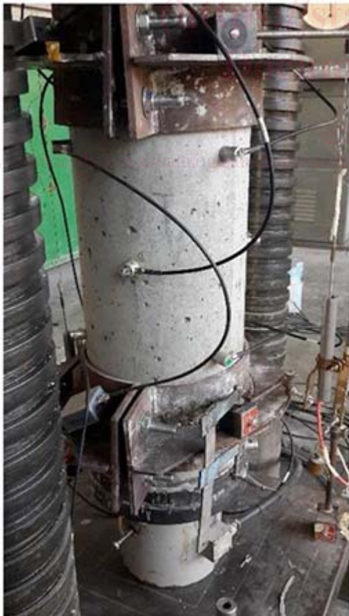
FIG. 2 Reinforced Column Specimen During Compression Testing
