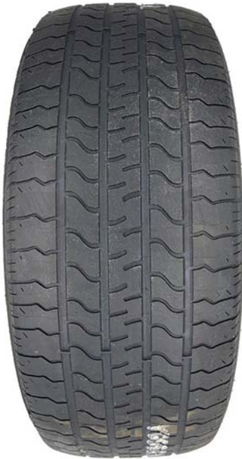
FIG. 1 Front View of the P225/60R16 97S Radial Low Tread Depth Standard Reference Test Tire
