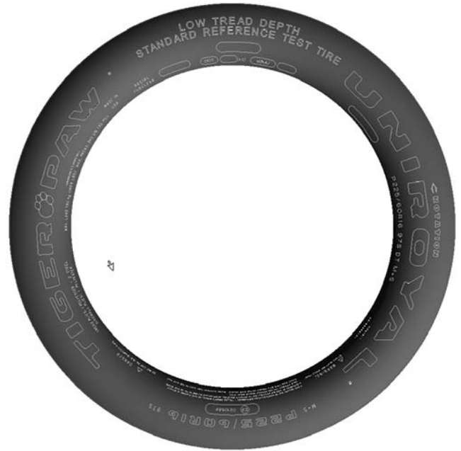
FIG. 2 Sidewall stamping of the P225/60R16 97S Radial Low Tread Depth Standard Reference Test Tire
