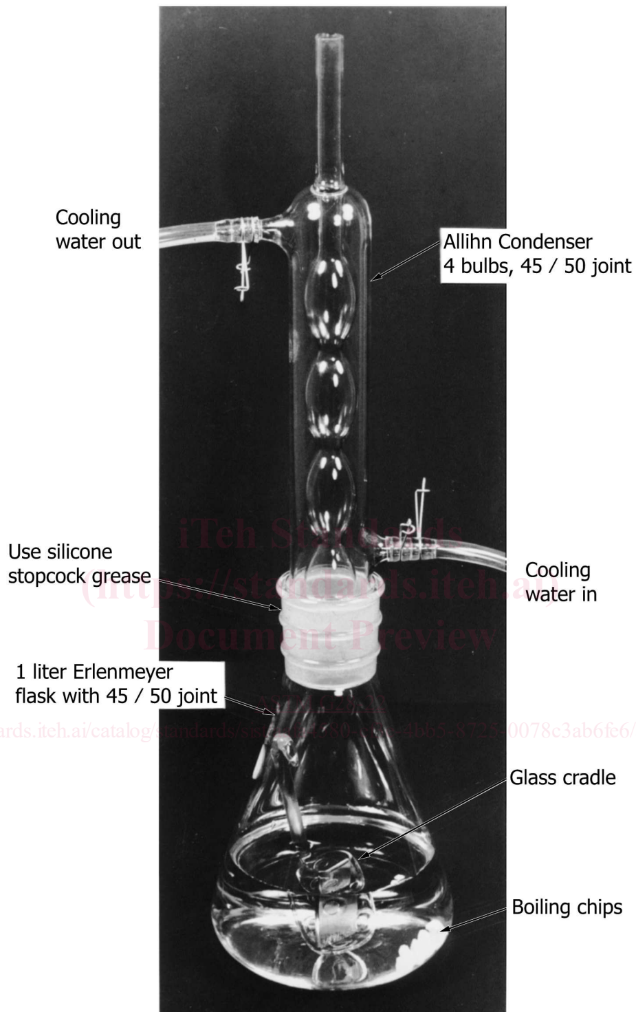
FIG. 1 Apparatus for Ferric Sulfate-Sulfuric Acid Test
