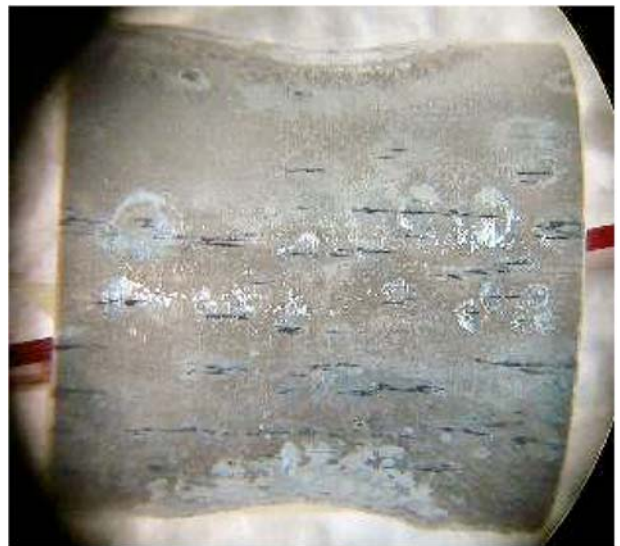
FIG. 2 Photograph Showing Example of Lined-up Pitting on C-ring Specimen
