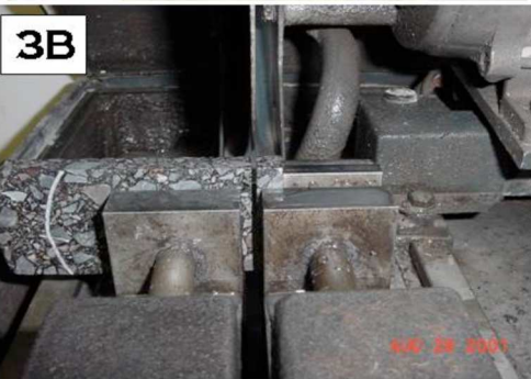
FIG. 3 Sample Preparation to Obtain 50-mm x 50 mm Wide by 12-mm x 12 mm Wide by 10-mm x 10 mm Thick Specimen-Specimen
