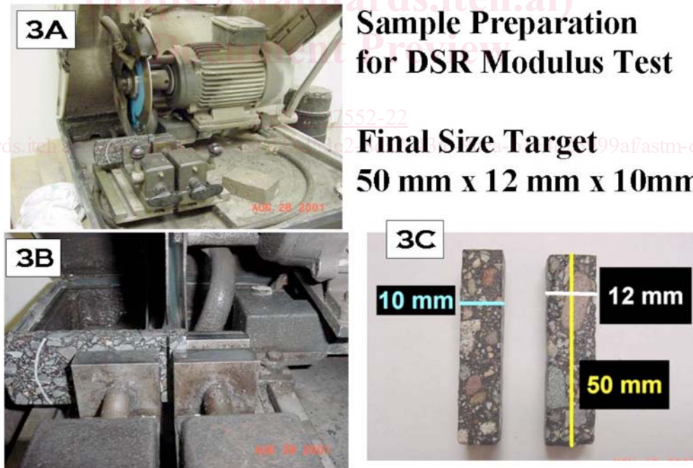
FIG. 3 Sample Preparation to Obtain 50 mm Wide by 12 mm Wide by 10 mm Thick Specimen
