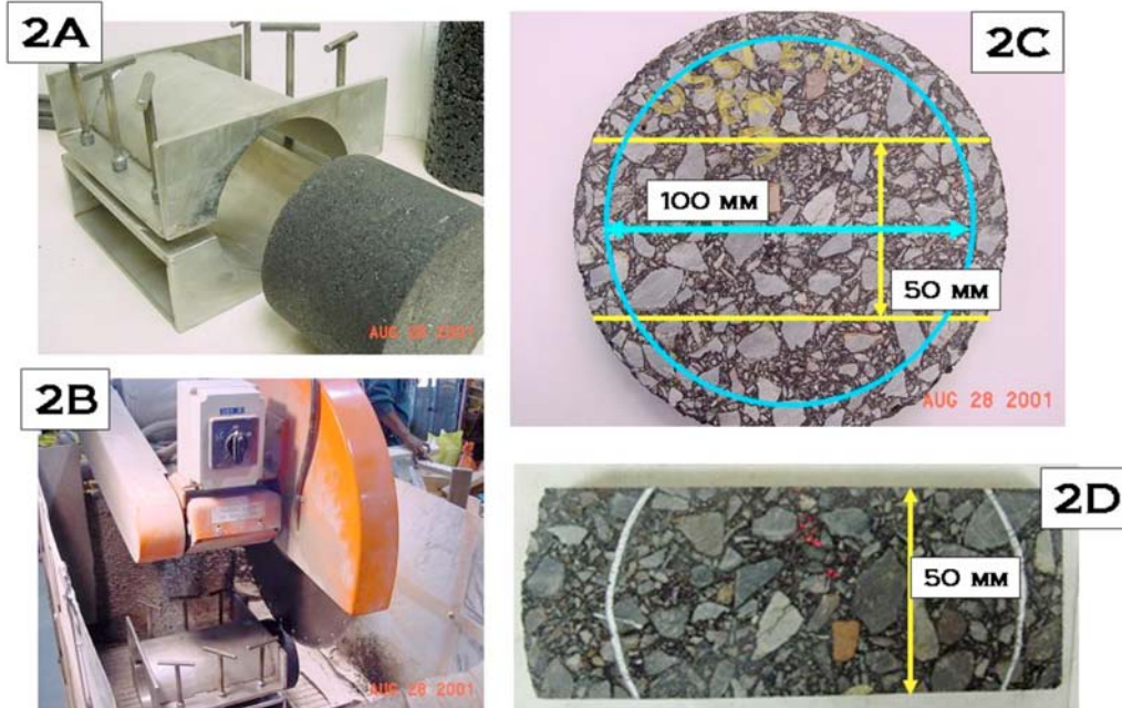
FIG. 2 Sample Preparation to Obtain 50 mm Wide by 12 mm Thick Rectangular Specimen
