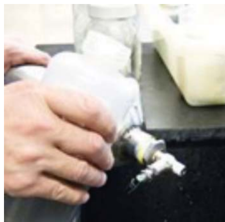
FIG. 9 Soap Water Solution Leak Testing
