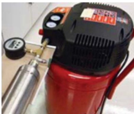
FIG. 8 Filling the RPV with Compressed Air
