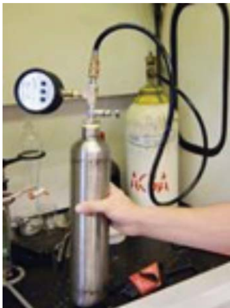
FIG. 7 Connecting to the SO 2 Filling Hose
