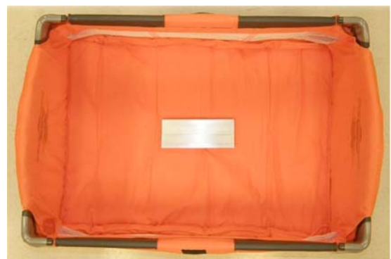
FIG. 3 Test Mass Positioned for Bedside Sleeper Accessory Sleep Surface Test
