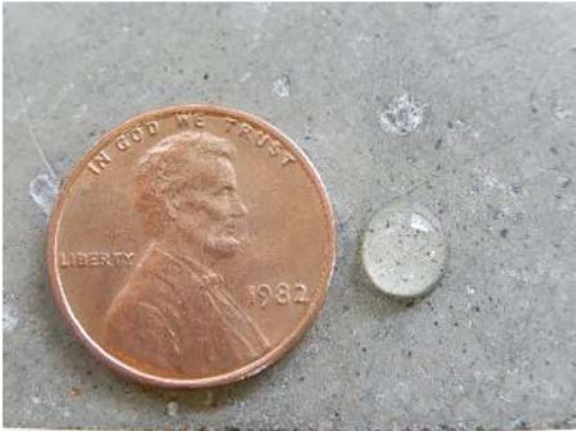
FIG. 1 Non-absorptive Concrete Surface
