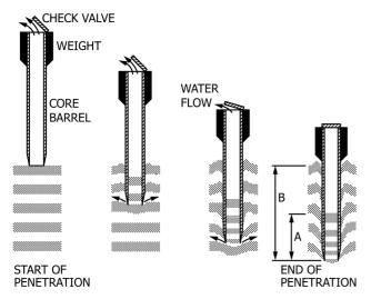
Note 1—Dark bands represent stiff sediments; light bands represent plastic sediments. As coring proceeds, sediment below the barrel moves laterally away from the cutting edge and plastic sediments inside the barrel are compressed. "A" is the core's length and "B" is the barrel's penetration depth.
