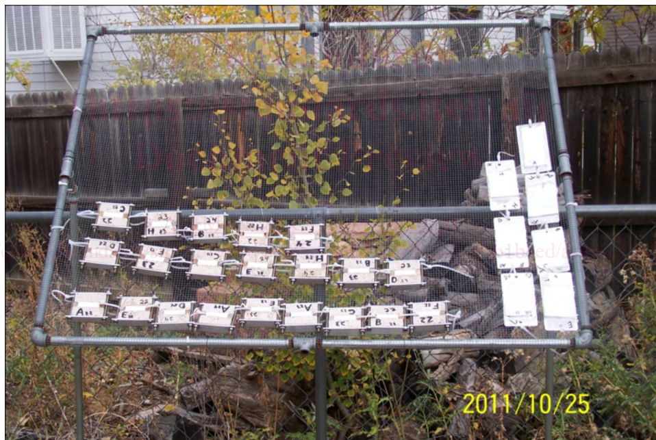
FIG. 5 Specimens Attached to Test Rack
