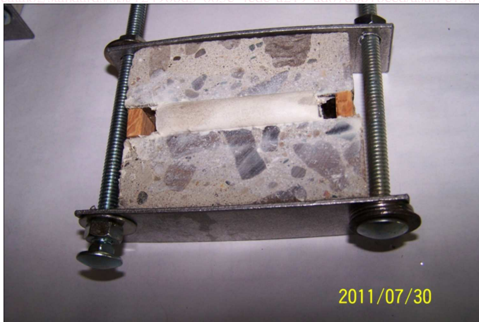
FIG. 3 Clamping Device Holding the Specimen in Compression
