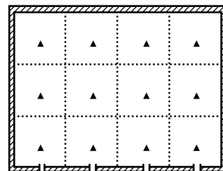
FIG. 1 Traverse Positions for Rectangular Flue
