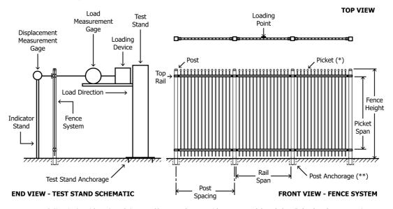
\* Note 1 - Any picket point style is acceptable on tested system; pickets may extend through the rails (as shown) or may terminate at the rails. Range of qualification is based on maximum picket span. \*\*Note 2 - Anchorage should be to concrete surface using core-drilled holes filled with grout or welded base plates and anchor bolts.
