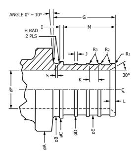
Note 1—All dimensions shall be measured with appropriate micrometers, such as pin or ball micrometers for wall thickness, and outside-diameter micrometers with flat anvils, or vernier calipers, to measure outside diameter and width of cold-expansion fittings and compression-sleeves.
