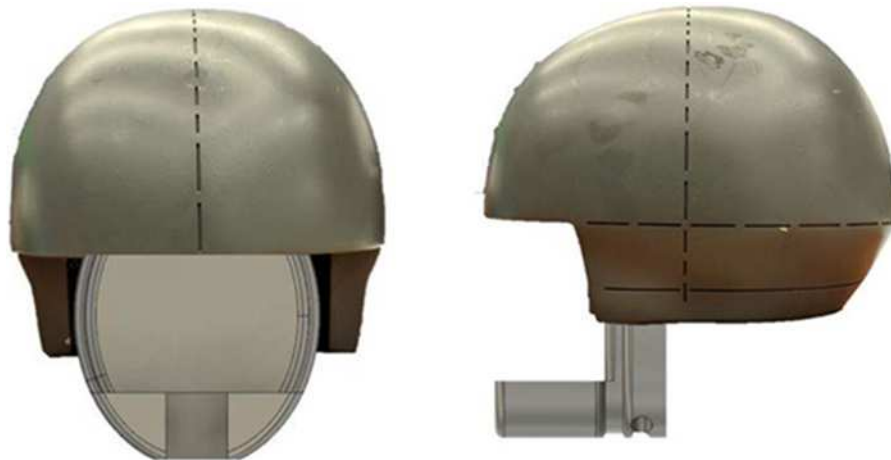
FIG. 3 Example Headform with Chin Strap Attachment Point
