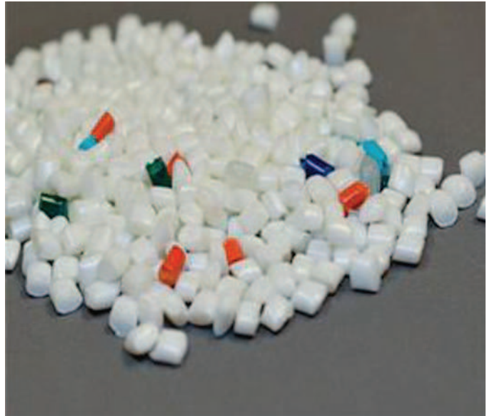
FIG. X1.8 Polymer Cross-contamination (The example shown relates to contamination by colored pellets.)
