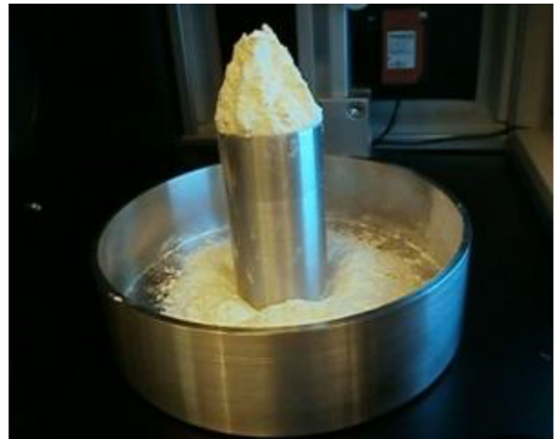
FIG. 2 Apparatus to Determine Angle of Repose
