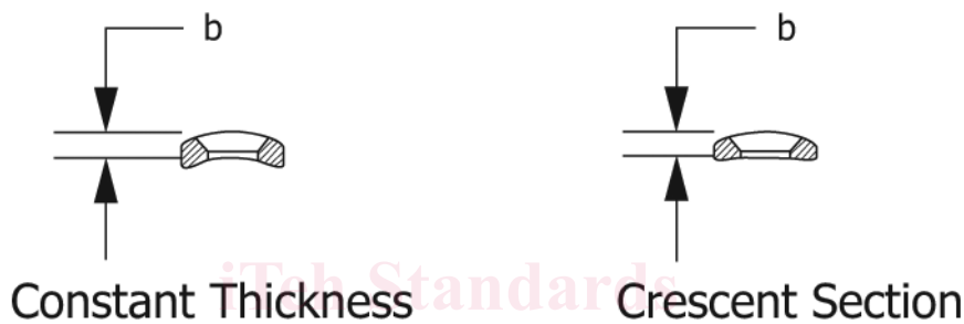
FIG. 3 Bone Plate Cross Sections
