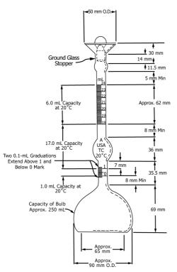
Note—Variations of a few millimetres in such dimensions as total height of flask, diameter of base, and so forth, are to be expected and will not be considered sufficient cause for rejection. The dimensions of the flask shown in Fig. 1 apply only to new flasks and not to flasks in use which meet the other requirements of this test method.
