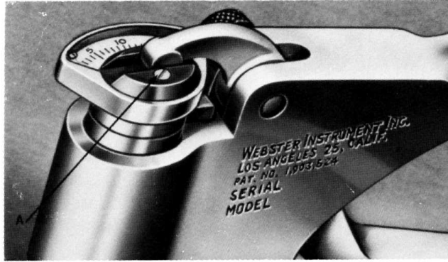
FIG. 3 Zero Adjustment Screw, A (indicated by arrow)
