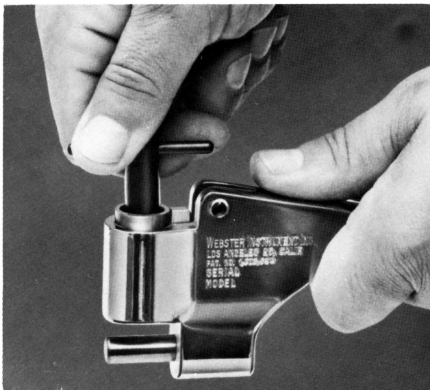
FIG. 4 Adjusting Load on Load Spring
