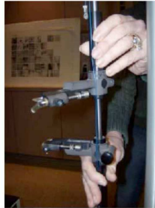
b. Photograph of Cable "Roller Style" Extensometer
