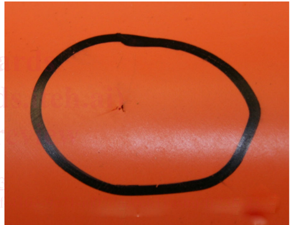
FIG. 5 Breakdown (Dielectric Failure Blanket: Front)
